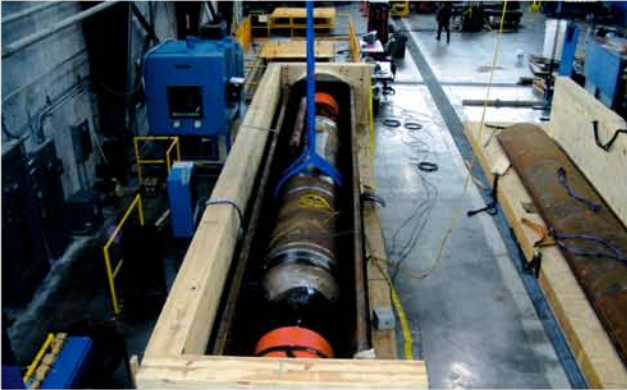
A cylindrical test sample is placed in the safety enclosure inside the environmental chamber.
