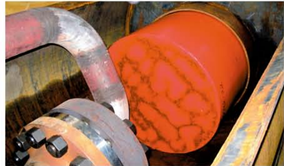
A view of the flanged end of a test vessel and the energy absorbing bumpers.
