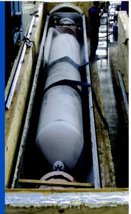
A view of the flanged end of a test vessel and the energy absorbing bumpers.
